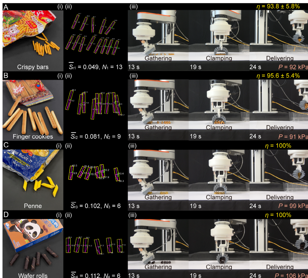
Figure 7. Soft gripper inspired by the gripping fashion of an elephant trunk tip for transporting scattered granular food. A) Crispy bars. B) Finger cookies. C) Penne. D) Wafer rolls. i) Scattered granular food with varying granularities and quantities. ii) Edge detection of the granular food. iii) Snapshots of the transporting process.
